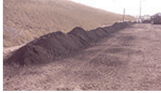
Undercutting ballast tailings Enlarge
