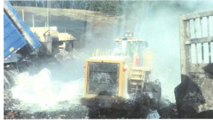
Deposition of white solids on dozer. Plume moving up and to right. Coffin Butte Ridge evident in top left of photo.
