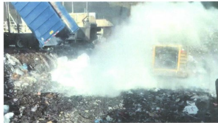
Plume of particulates forming near and above compacting dozer.
